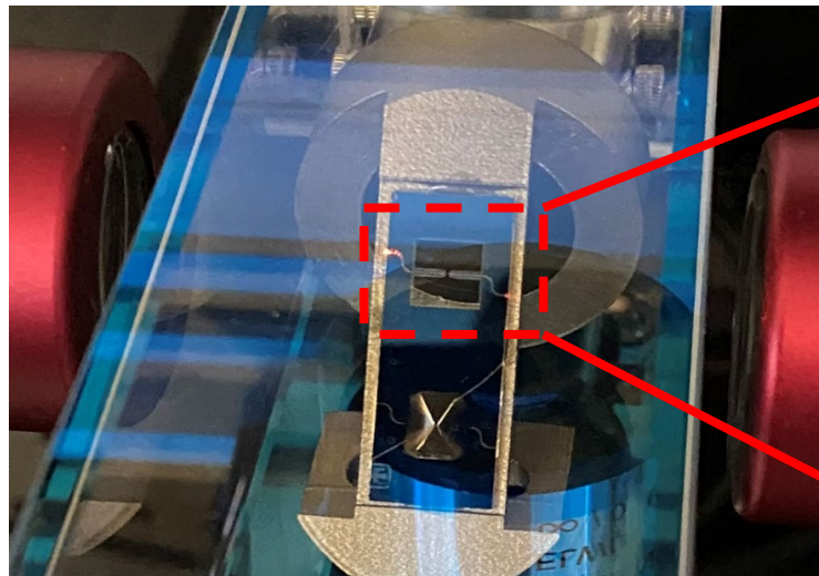
Light-coupled waveguide via high NA objectives
