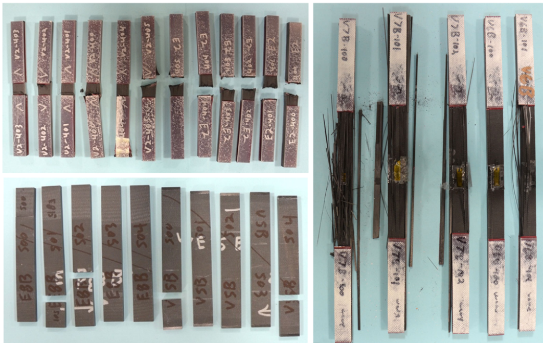
Figure 9: Post-Structural Testing Specimens: compression (top left), transverse tensile (bottom left), and longitudinal tension (right).
