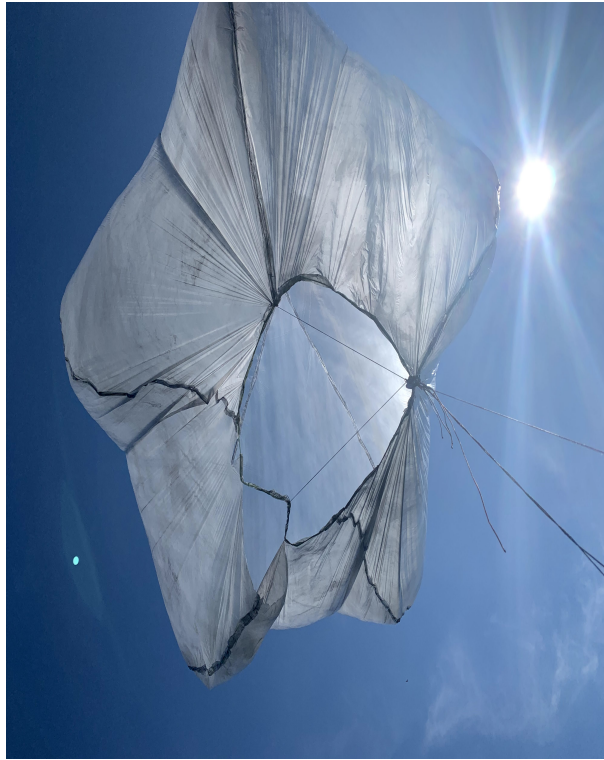
Fig. 7 Ripped Envelope During Tethered Solar Balloon Experiment
