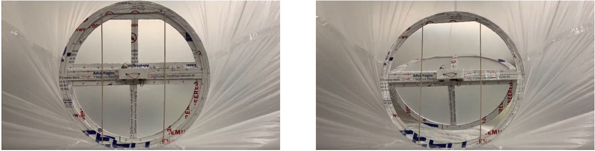
Fig. 9 Flapping Vent in Closed and Open Configuration (Top-Down View)
