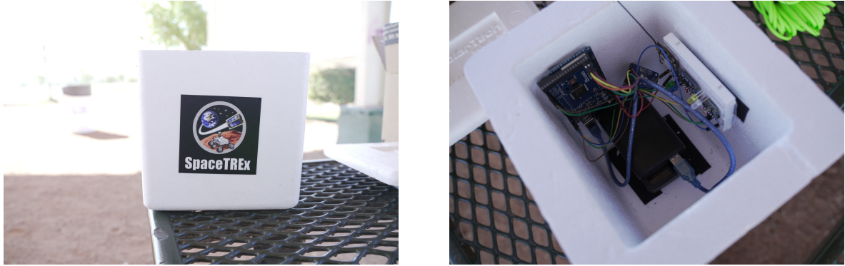
Fig. 4 SHAB Styrofoam Gondola with Internally Mounted Electronics
