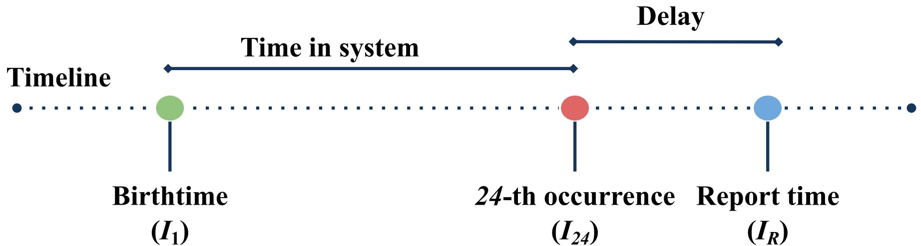
$$\text{delay} \leq \alpha * \text{time in system}$$
