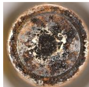
Figure 4. Close-Up Photograph of Honda Accord Injector Tip
