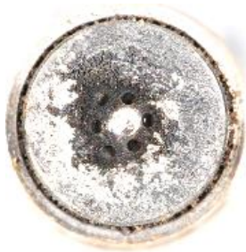
Figure 5. Close-Up Photograph of Honda Civic Injector Tip
