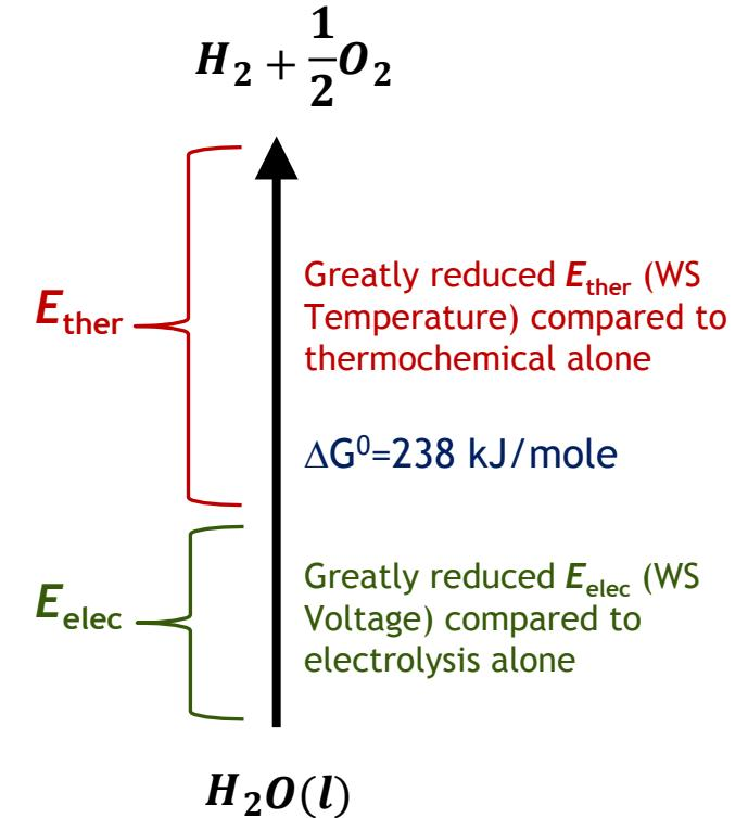
Interplay between temperature and electrochemistry allows us to tailor the hybrid cycle to particular thermal source
