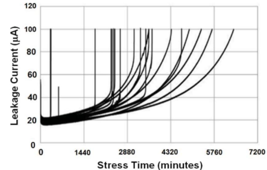
Accelerated test (5x  $V_r$ )
