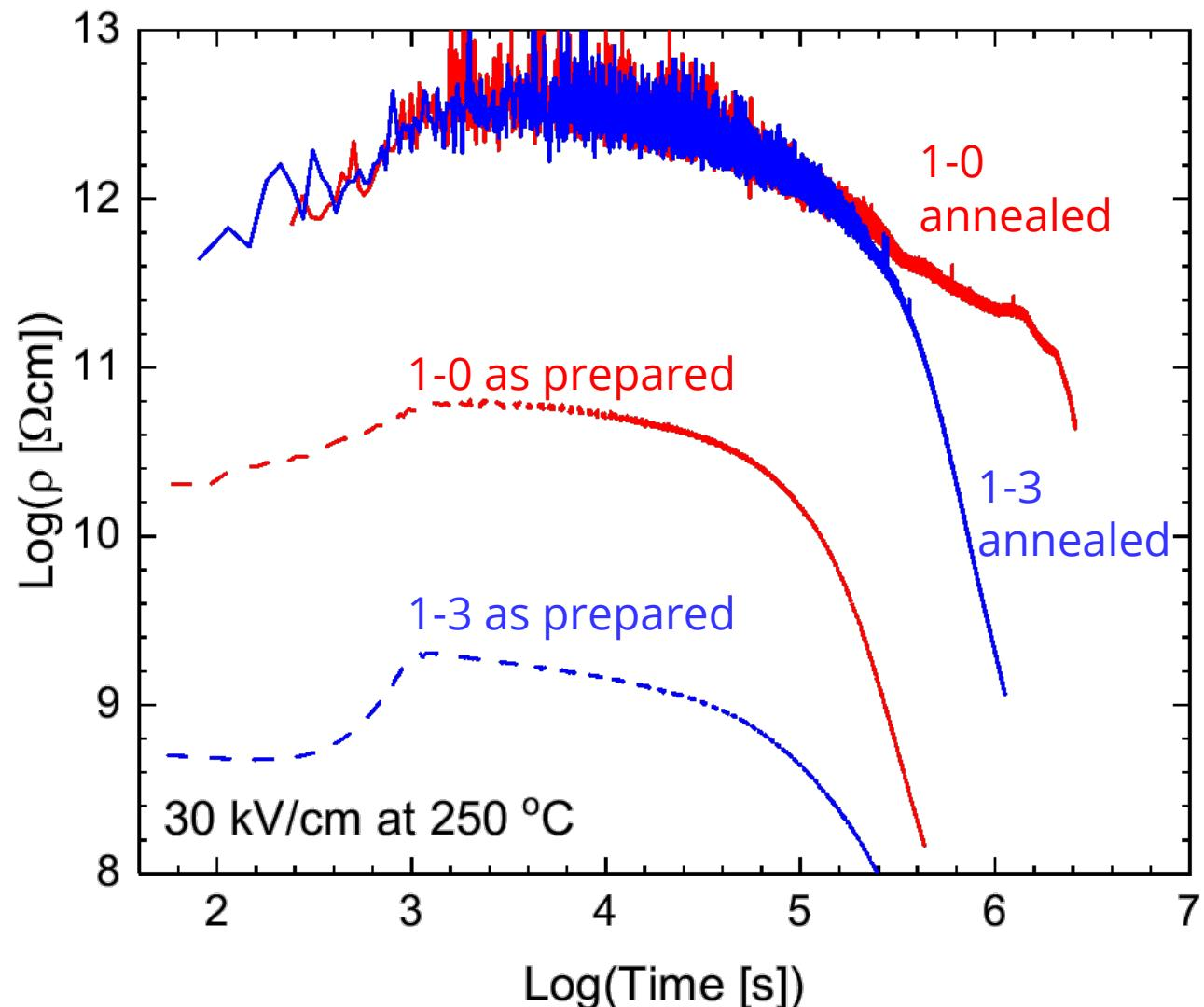
→ Sintering in air may cause high  $[\text{V}_0^{**}]$ , reducing DC lifetime
