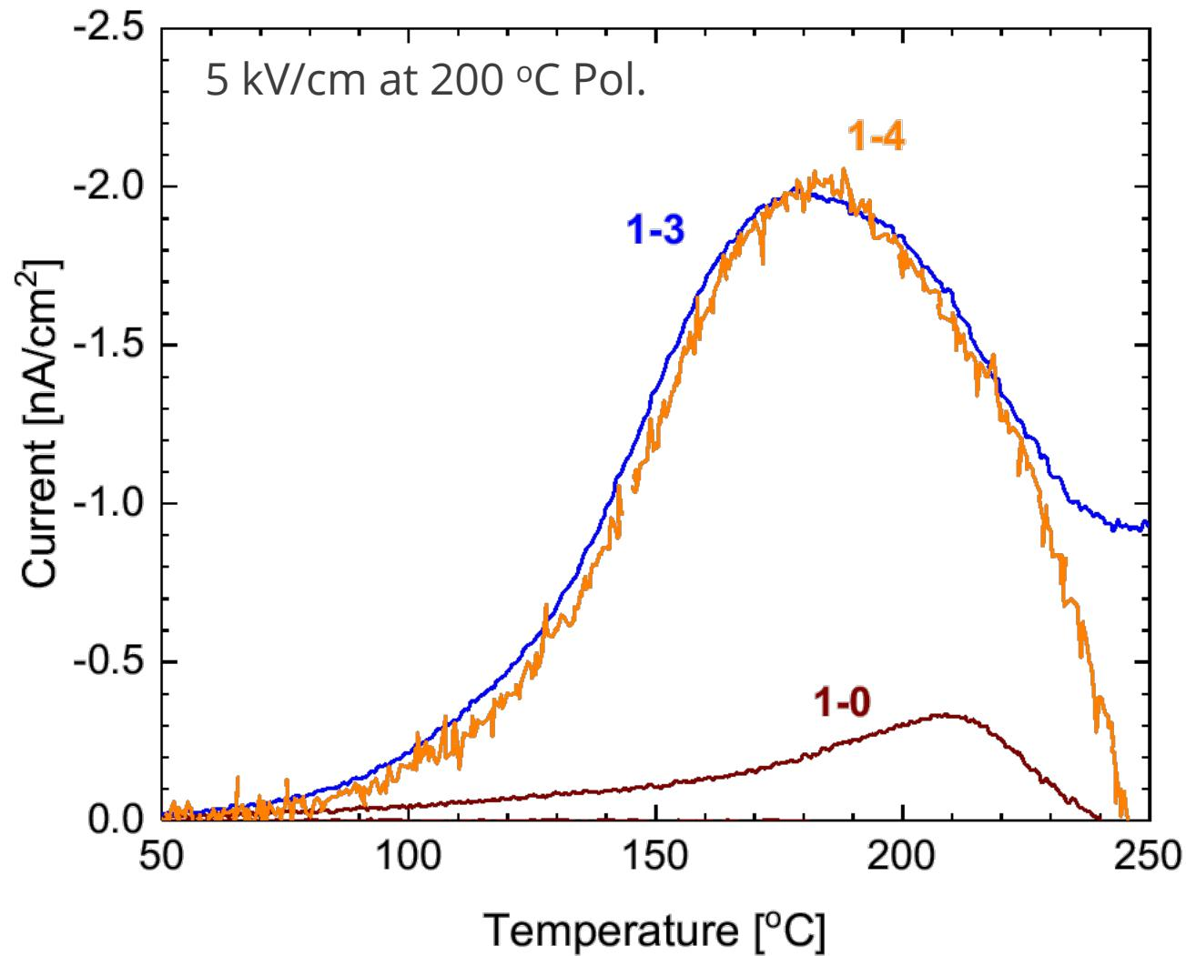
Very large TSDC near center of sample, consistent with significant  $V_{\text{O}}^{**}$  concentration
