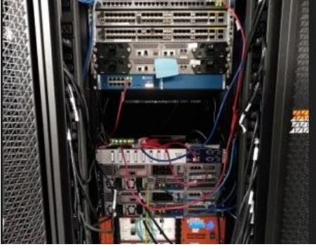
Fig. 3: QNET conventional node Dave consists of two supermicro Linux hosts, two Cisco 3064 switches and a Polatis all-optical switch.
