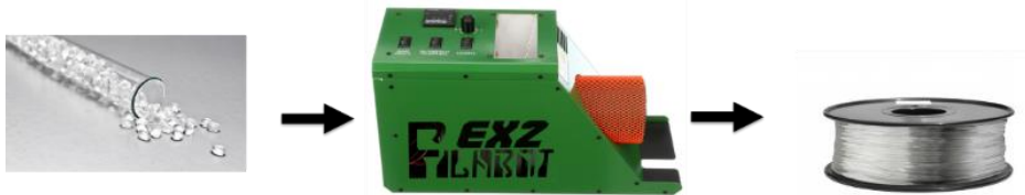
Figure 5. A visualization of the filament extrusion process. First, polymer pellets are loaded into the extruder. The extruder melts the polymer and extrudes it at a controlled diameter to make 3D printable filament. Photos adapted from [6-8].
