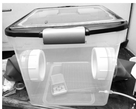
Fig. 2. Argon shower box with glove inserts.
