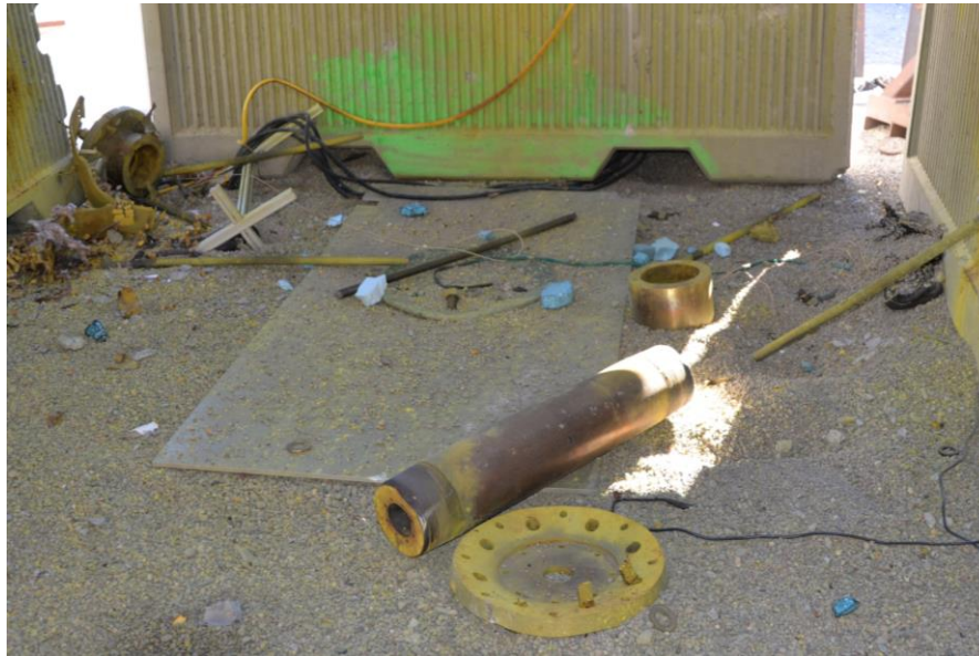
Figure 5. DDT tube after LLM-105 formulation nominal density thermite ignited test
