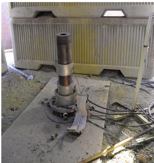
Figure 4. DDT tube after LLM-105 formulation nominal density slow cookoff test
