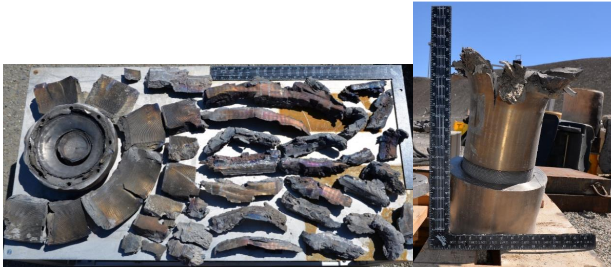
Figure 6. Fragments of the LLM-105 formulated molding powder pour density DDT tube
