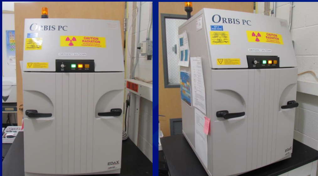
Orbis PC used for X-Ray Fluorescence (XRF) Mapping
