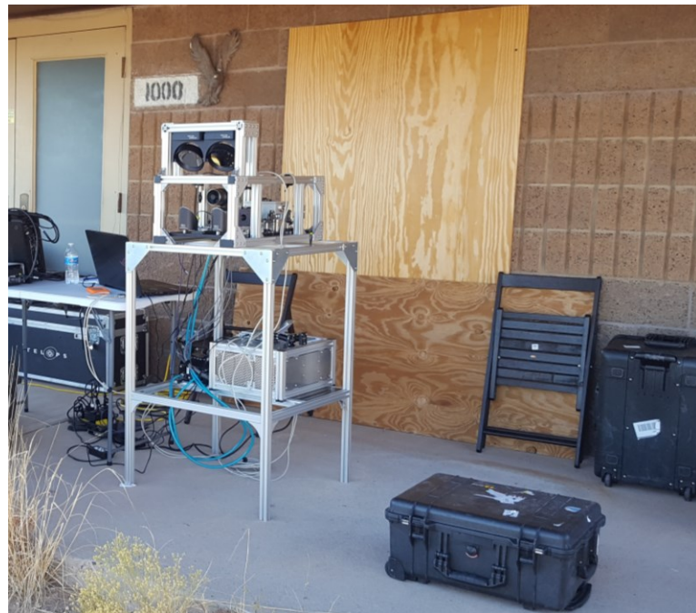
Figure 2: Photograph of swept-ECQCL remote detection system located at EMRTC “Little Eagle” site.
