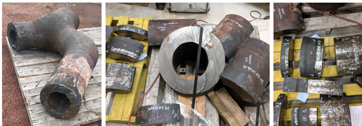
Figure 20. Photographs of the Wye Block section from the dismantled plant and during sample sectioning for the weld test sections.
