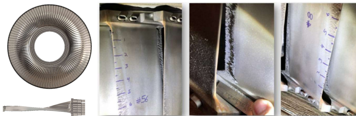
Figure 1. Images of the series of blades in question. The pitting of the trailing edges of the blades can clearly be seen in the higher resolution close-up images.
