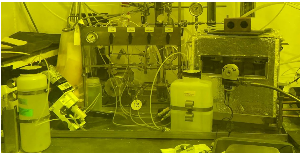
Figure 3.2. Ion Exchange Assembly in the Hot Cell
