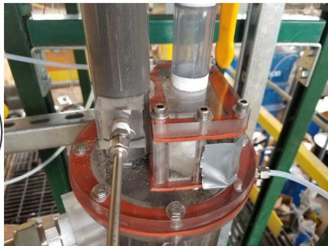
Figure 8 Biomass Injection Port at the Top of the Reducer
