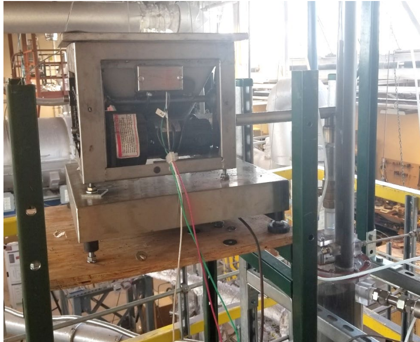
Figure 7 Screw Feeder for Biomass Injection
