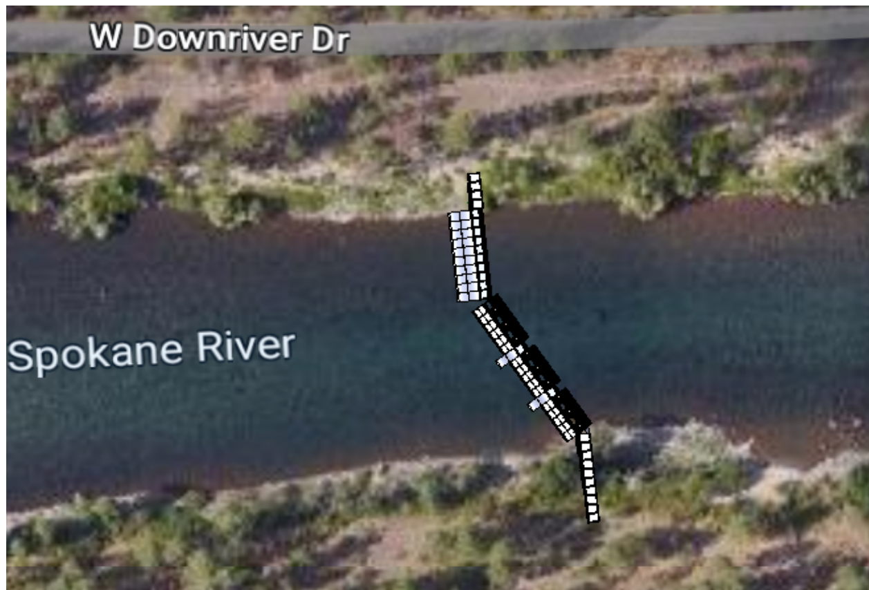
Figure 38: Plan view of the 3D SolidWorks model of the LPS 566 facility overlaying a Google Map image of the site location on the Spokane River. Flow is from right to left.
