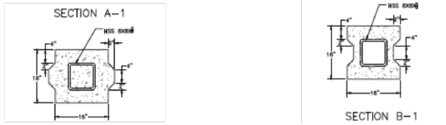
Figure 13: Bottom grade beam, weight equals 6 tons.
