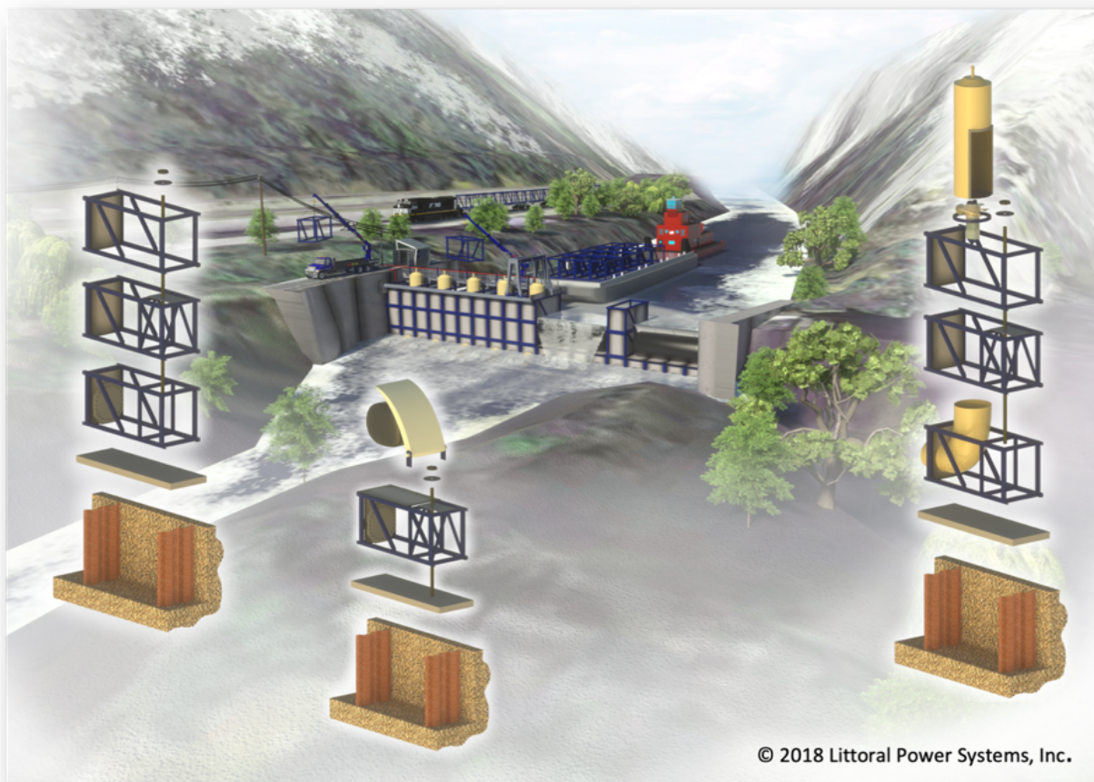
Figure 2: First generation h-Modular facility including the module stack types at the start of the project. Flow direction for the expanded module stack images is from right to left.
