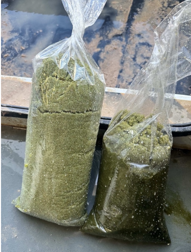
Figure 16. AFM ® filtration media used after the dissolved air flotation process.
