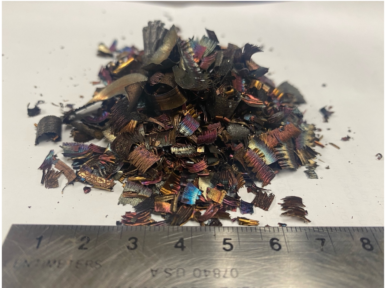
Figure 15. Ferrous machine shop turnings used in the scrap iron tank.
