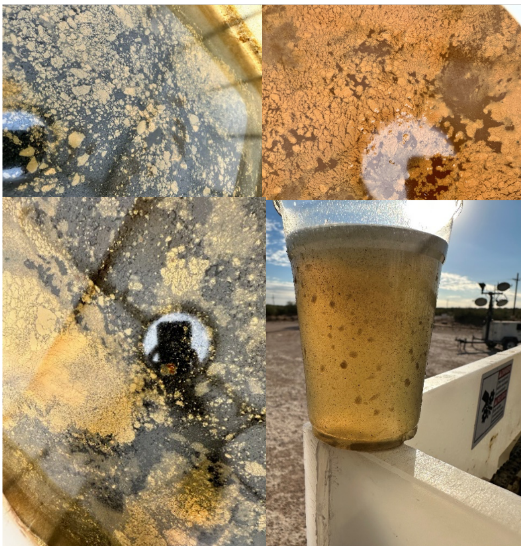
Figure 20. Congealed hydrocarbons floating in clear wells on November 15, 2022.
