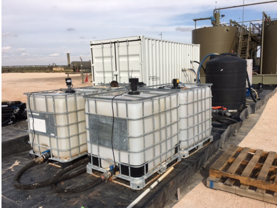
Figure 2. Equipment set-up at field test site. Four clear wells are shown in foreground. Product water from the treatment system was collected in a 500 gallon polyethylene tank.
