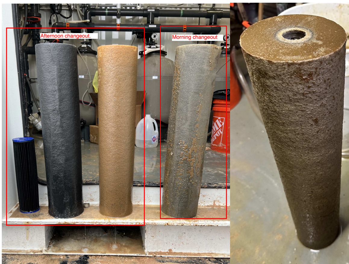
Figure 19. Clogged cartridge filters on November 19, 2022. Cartridge filters prevent particulates from entering the electrochemical cell.
