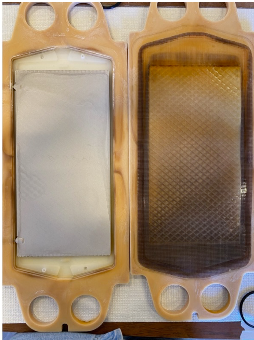
Figure S3. Cathode and cathode facing membrane after 2 hours of operation at a current density of 100 mA/cm 2 using feed water with the composition given in Table S1. No cleaning cycle was used in this experiment.
