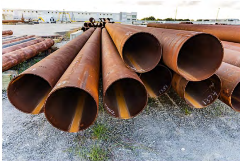
Figure 4—20" pipes to be treated in the application trial.
