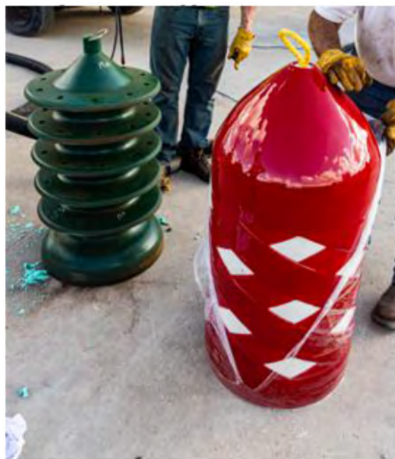
Figure 5—Pigs used for treatment application in pipelines.
