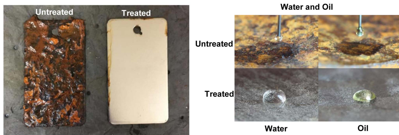
Figure 3—Results of salt fog corrosion testing for treated and untreated coupons. The omniphobic treatment is corrosion resistant and remains hydrophobic and oleophobic even after significant exposure.
