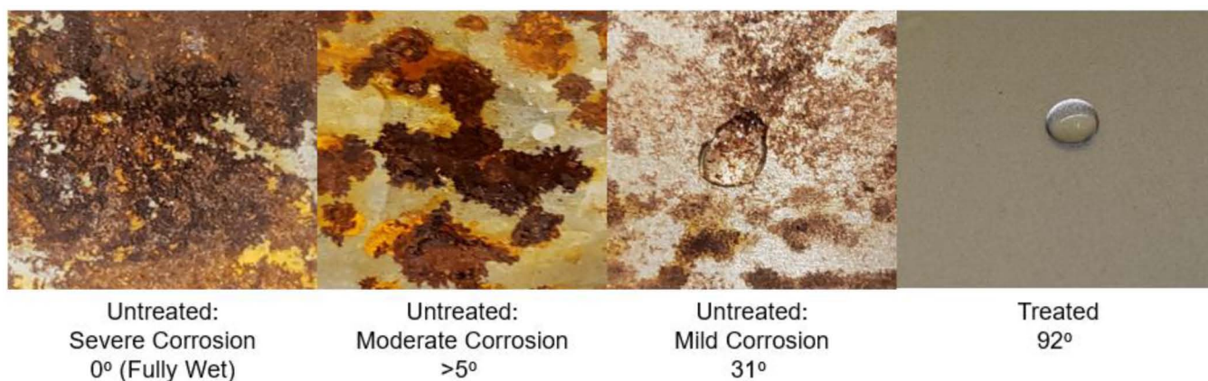
Figure 6—Water droplet wetting on various surfaces: untreated with severe corrosion, untreated with moderate corrosion, untreated with mild corrosion, and treated.
