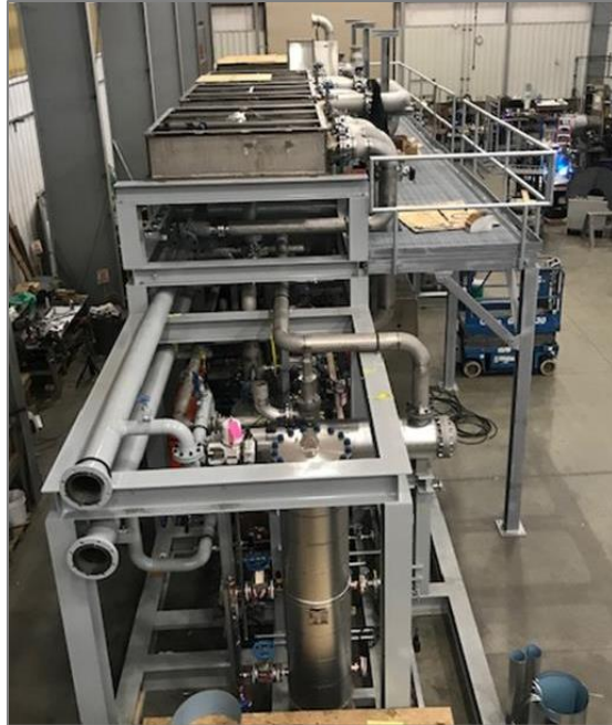
Figure 17. A view of the second level of the MTR test system with the membrane module stack bases visible prior to installation of the modules.
