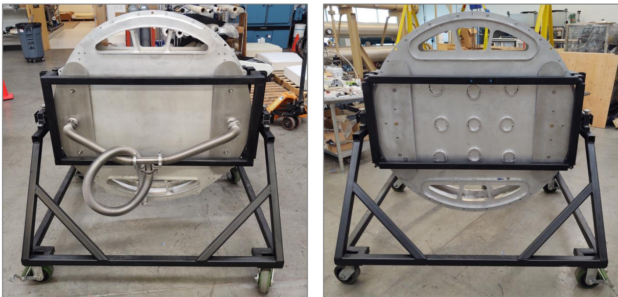
Figure 9. Front (left) and back (right) views of the MTR leak test apparatus for the TCM field test membrane modules.
