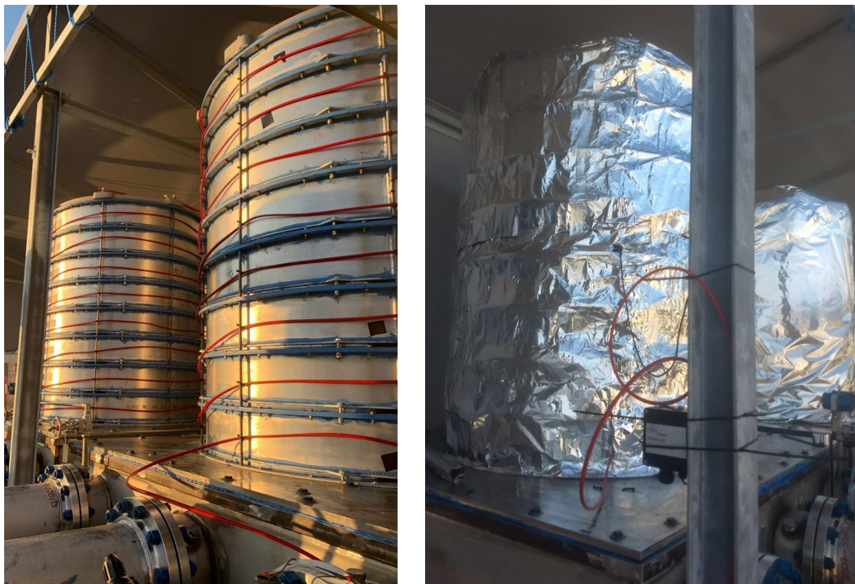
Figure 28. 1 st Stage membrane stacks with heat trace (left) and insulation (right) installed.
