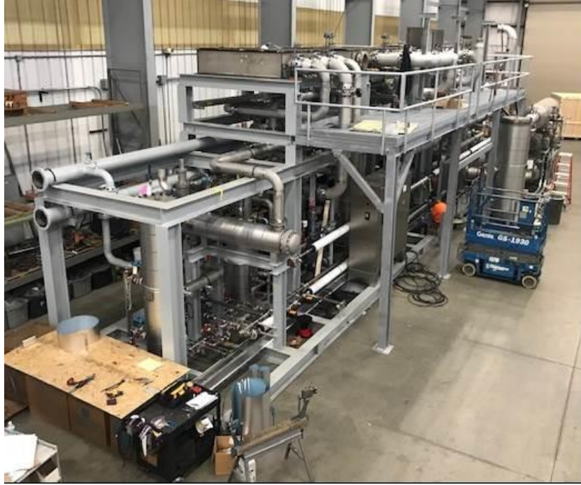
Figure 16. An early isometric view of the MTR test system at PRI. The first floor contains the blowers and pumps used to move gas through the system, while the second floor will hold the membrane module stacks.
