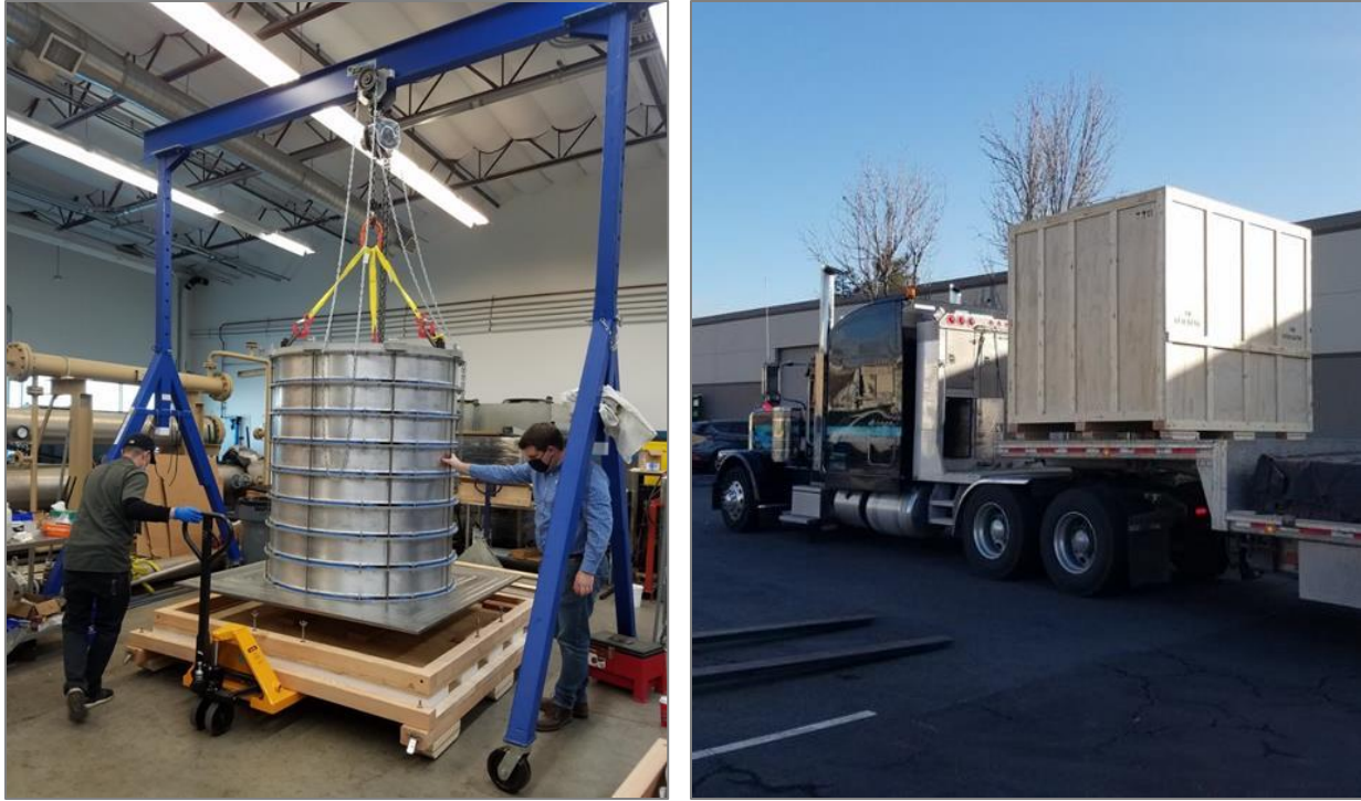
Figure 10. Packing of the MTR advanced membrane module stack and lid at MTR (left) and crated stack ready for transport to fabrication shop (right).
