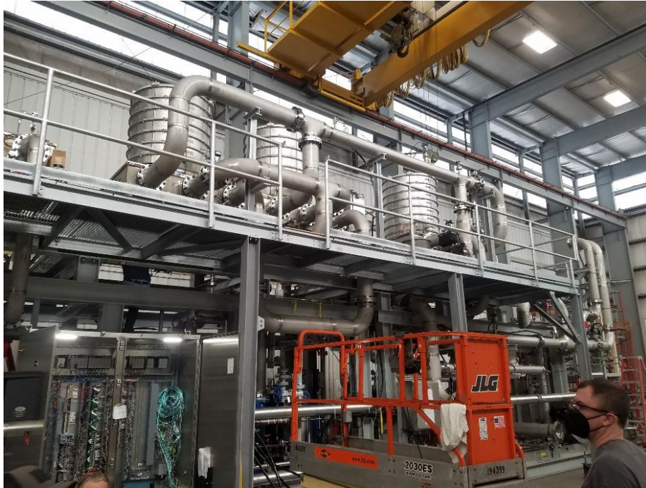
Figure 19. Picture of the membrane module stacks installed on the second floor of the test system at the PRI fabrication shop.
