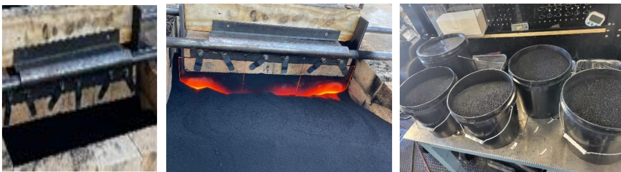
Figure 20. Semi-automated Flash Joule Heating reactor with carbon black substrate (left and middle) and graphene product (right)
