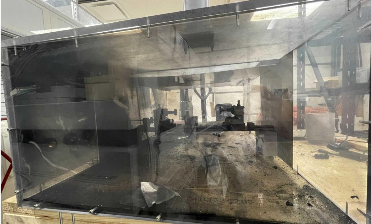
Figure 7. Flash Joule Heating chamber at Universal Matter’s Houston Innovation Center
