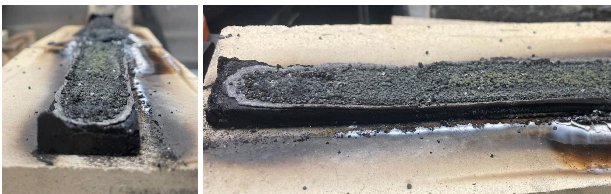
Figure 22. Sacrificial layer (molding sand) of Flash Joule Heating reactor after experiment
