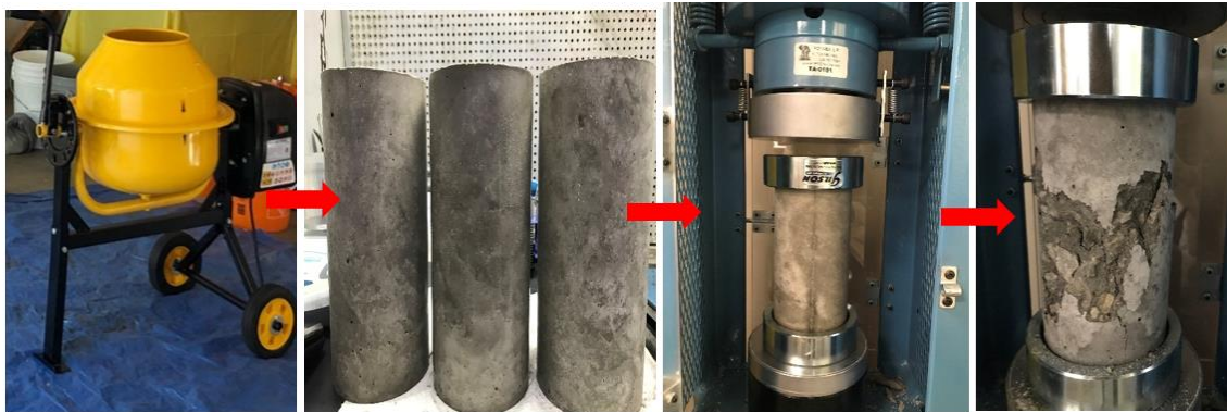
Figure 33. Photographs of concrete sample production (left), concrete samples (middle left), and sample testing (middle right, right)
