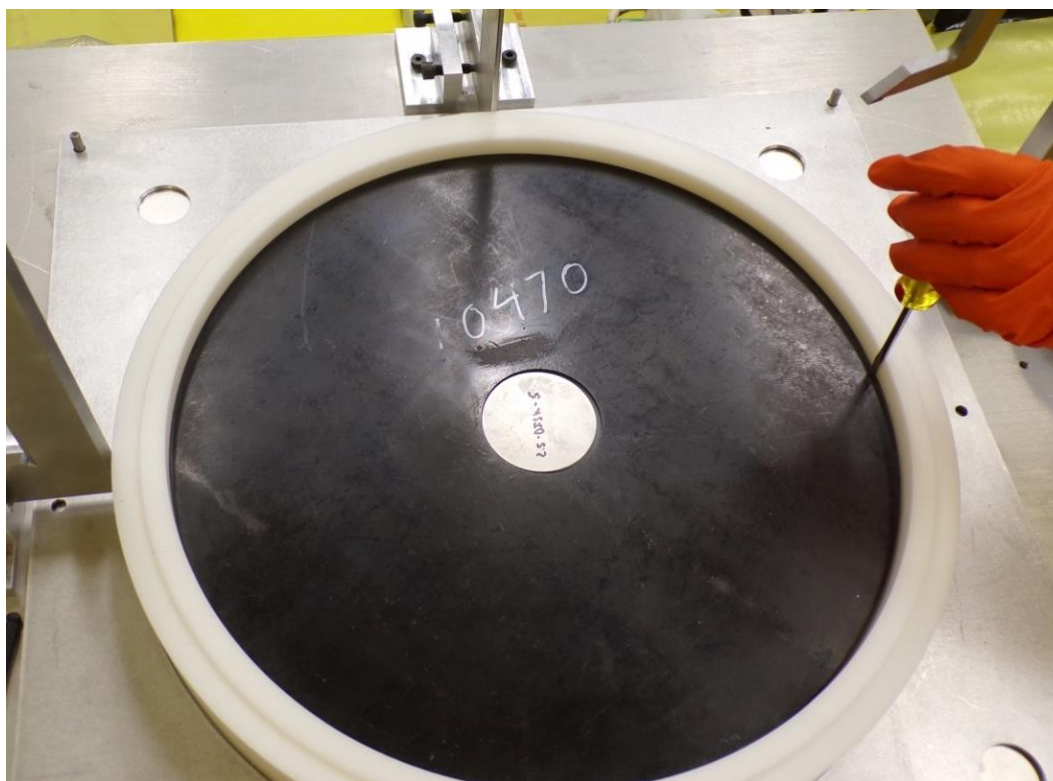
Figure 72. Experimenter positioning an HEU2 plate within the polyethylene reflector ring. Notice the 2.5" aluminum insert has also been pushed in the same direction.
