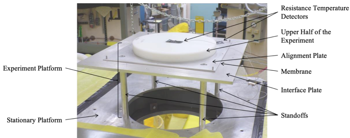
Figure 3. Upper stationary platform of the Comet machine, with the experiment platform.
