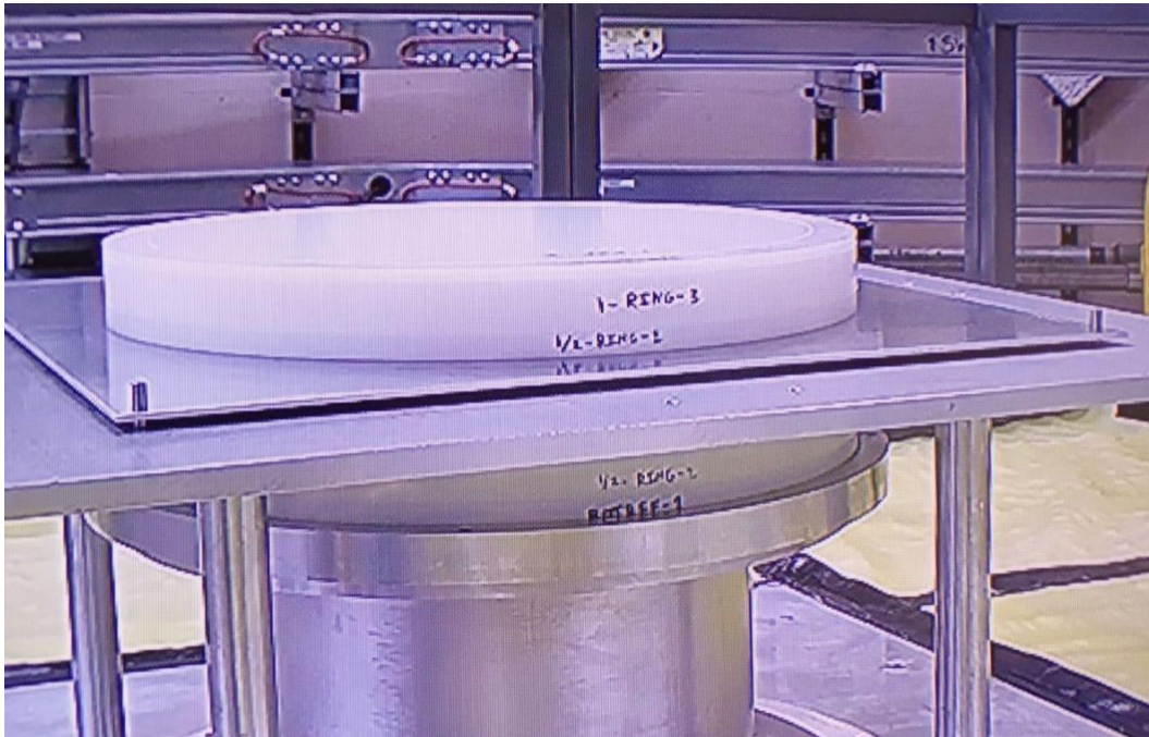
Figure 69. Fully assembled Case 3 experiment during operation (i.e., a photo of a critical nuclear reactor).
