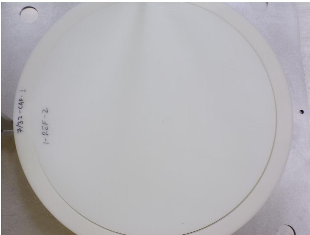
Figure 73. Upper half of the Case 3 configuration. Notice the crescent shaped gap on the right side of the 1-REF-2 part. This gap is from pushing the entire core stack to one side within the reflector ring.
