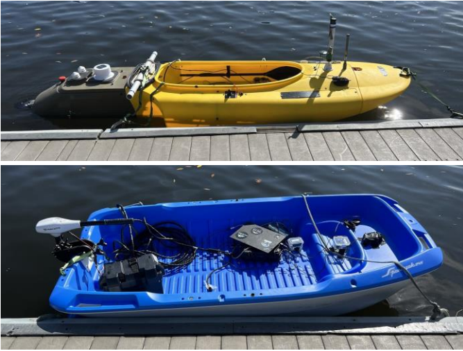
Fig. 2. The equipment used in our marine experiments. (Top) A Jetyak [66], which we refer to as a beacon, equipped with a GPS transponder. (Bottom) Standard watercraft, which we will refer to as Low-Nav craft, equipped with an electric trolling motor, Sparton AHRS-M2 attitude and heading reference system, and GPS transponder. Each platform has a MicroModem-2 [67] and acoustic transducer for inter-platform acoustic ranging and communications.
