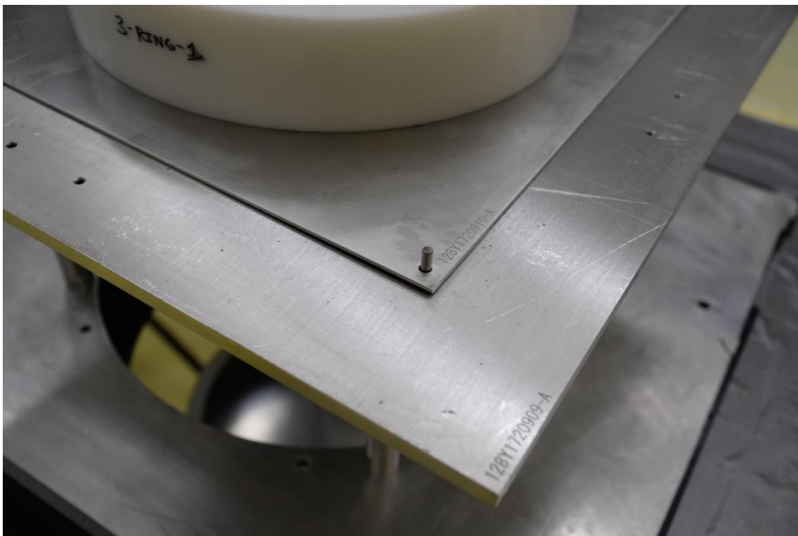
Figure 18. Membrane deflection under the weight of the 0" Std. upper stack.
