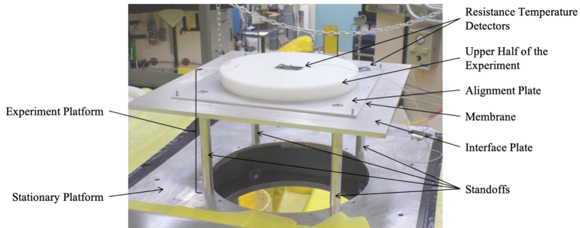
Figure 4. Upper stationary platform of Comet, with the experiment platform.
