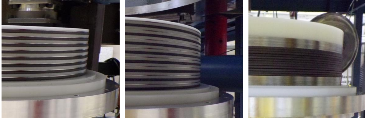
Figure 2. TEX-Hf stacking methods: Standard (left), Sandwich (middle), and Bunched (right).
