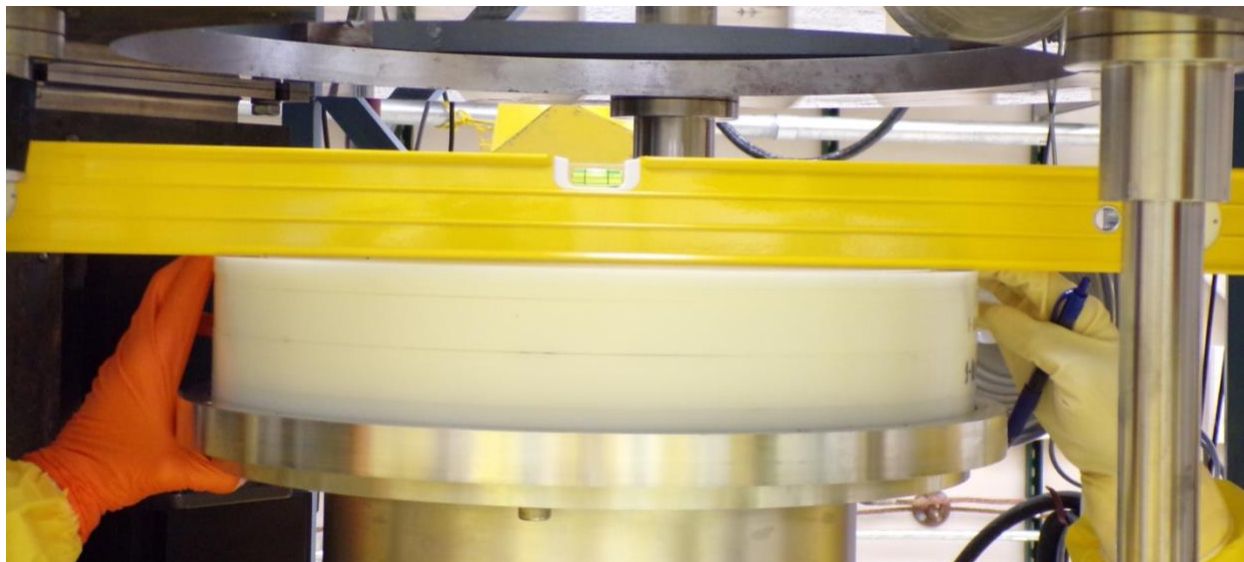
Figure 15. Levelness measurement for the lower core stack of 1/4" Std. using the bubble level.
