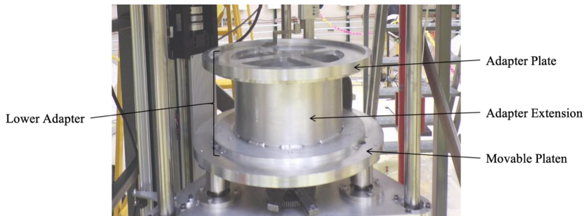
Figure 5. Lower movable platen of Comet, with the lower adapter.
