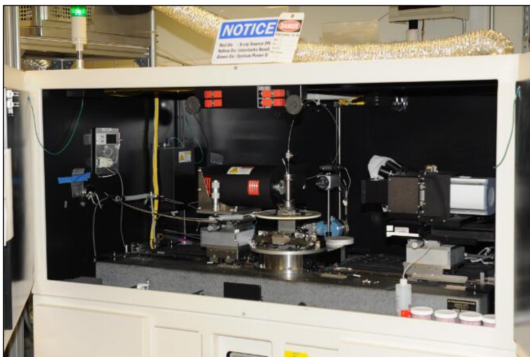
Figure 15: Zeiss Xradia MicroXCT-400 Micro-CT scanner used for high-resolution CT imaging at NETL.
