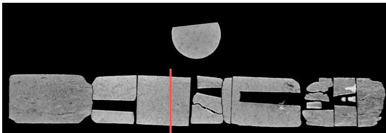
Figure 36: Single image from a video file available on EDX showing variation in the LG #1 core from 3,665–3,667 ft. Image above shows the variation in composition within the matrix perpendicular to the core length.
