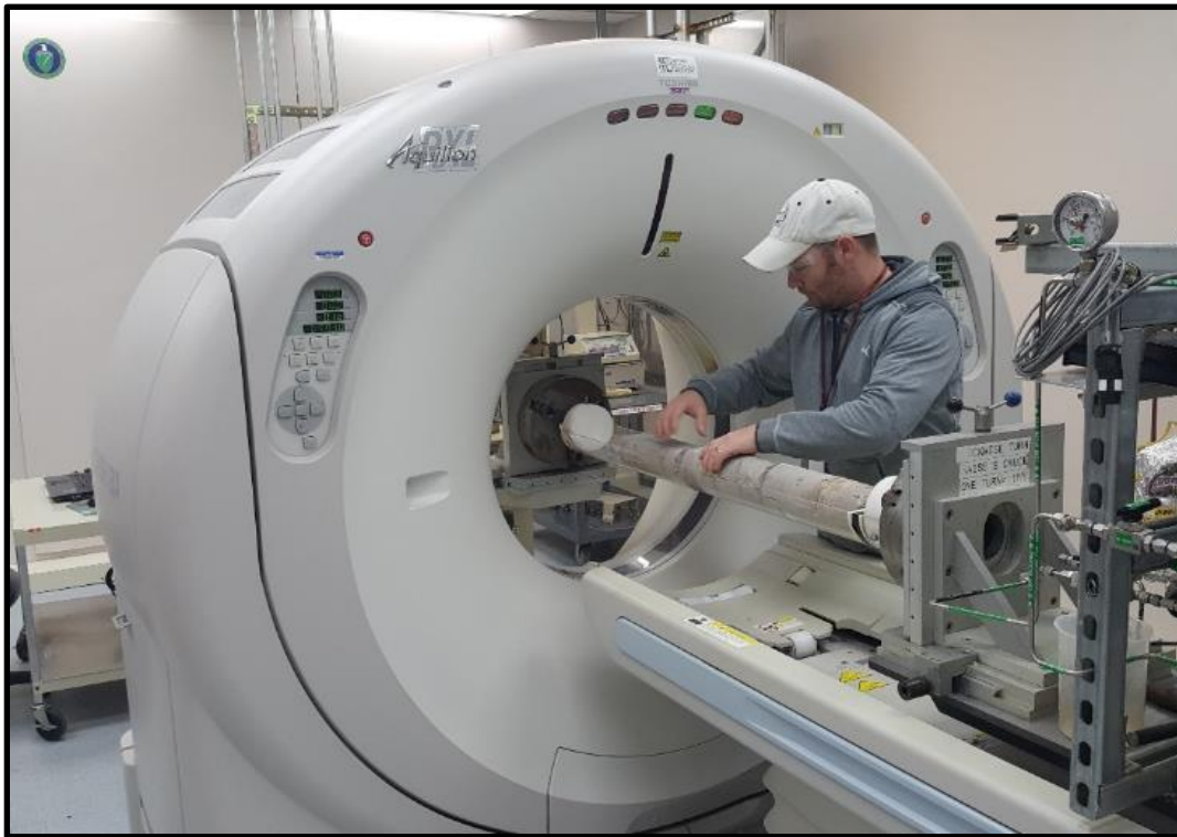
Figure 12: Toshiba Aquilion Multislice Helical CT scanner at NETL used for core analysis.
