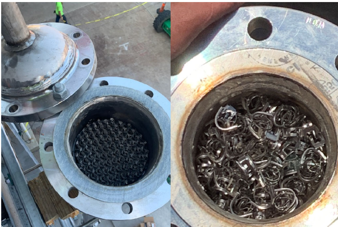
Figure 7-12. Absorber column (left) with Sulzer Mellapak™ 350Y structured packing and stripper column (right) with Koch-Glitsch IMTP® #15 random packing.
