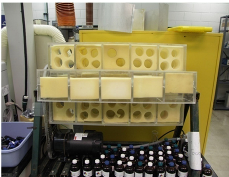
Figure 4-1. Photograph of a rotating tumbler used for activated carbon and ion exchange equilibrium measurements.
