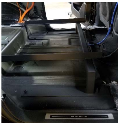
Figure 43: High and Low Voltage Wiring Showing New Components For DC Fast Charge Retrofit
