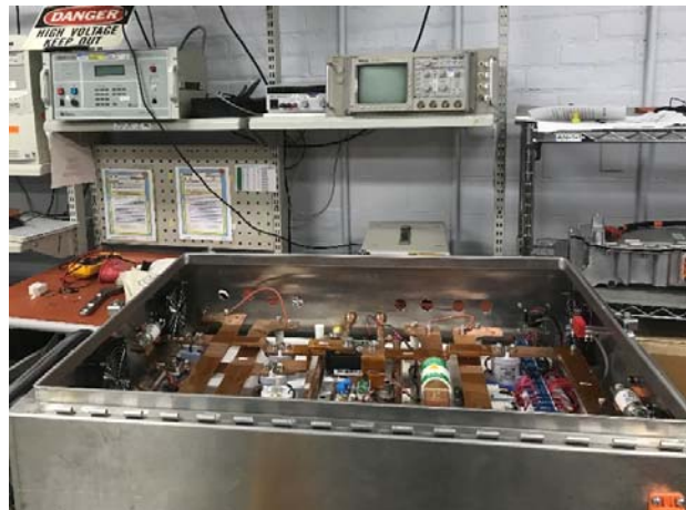
Figure 38: Withstand Voltage Test Setup
