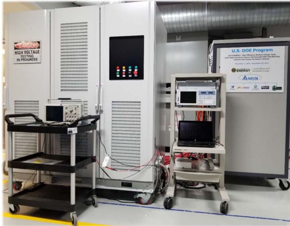
Figure I.1.1.6 1-Phase Series SST and Buck Module Test Setup (up to 45-kW)
