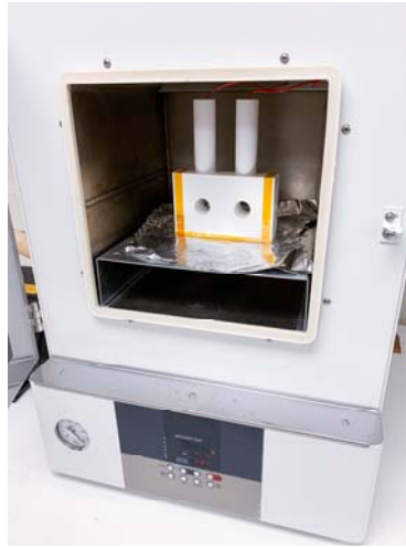
Fig. 26 Vacuum chamber for VPI
