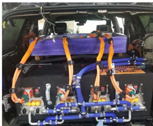
Figure 43: High and Low Voltage Wiring Showing New Components For DC Fast Charge Retrofit
