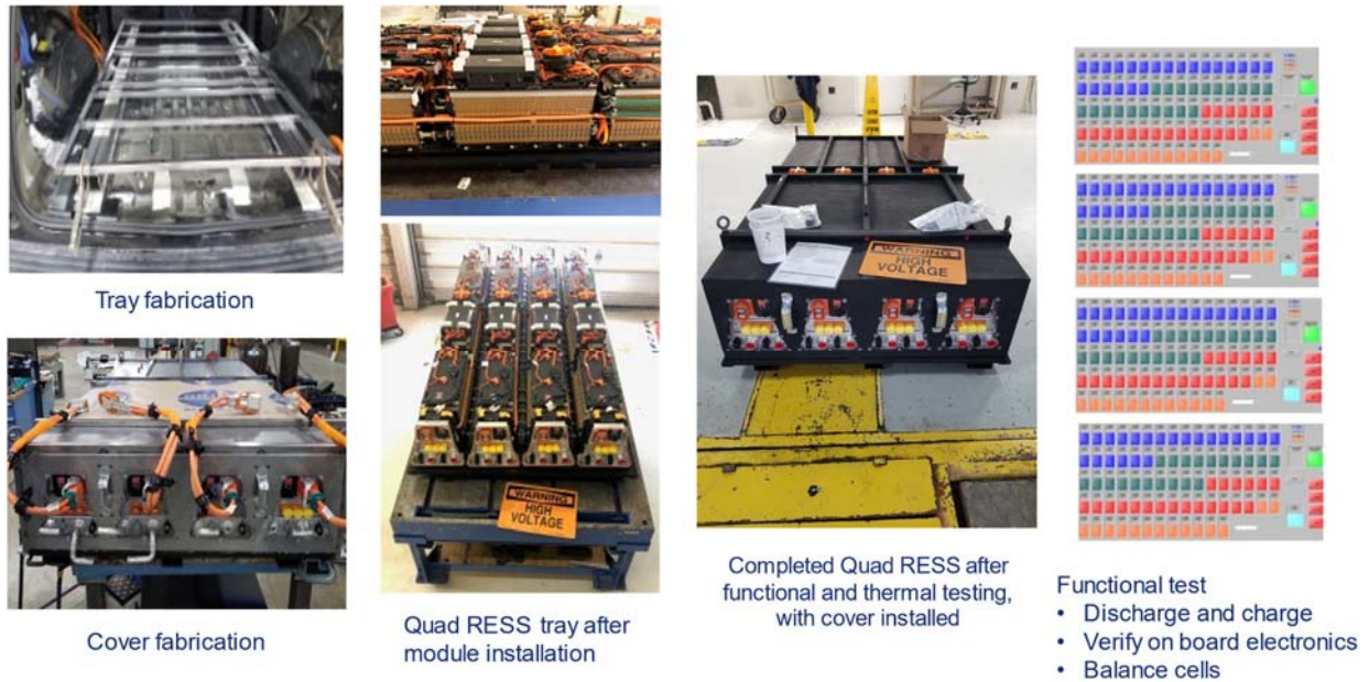
Figure 28: Stages of Quad RESS Build
