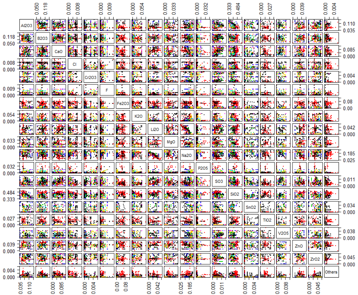
Figure 3.5. Scatterplot Matrix of 20 Components (mass fractions) for 691 LAW Glasses with Data for Normalized PCT Losses ( \text{g/m}^2 ) of B and Na that Remain after Excluding the 12 Glasses in Table 3.1
