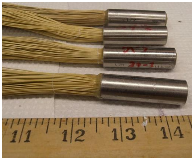
Figure 10. Potted hollow fiber membrane modules for lab test.
