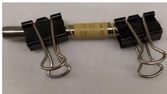
Figure 9. Macro-void-free fiber that wraps around a ¼-inch tube.
