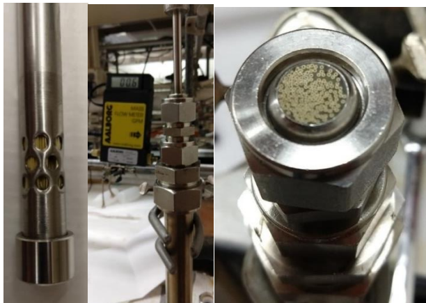
Figure 20. Leak-testing apparatus for fiber modules.
