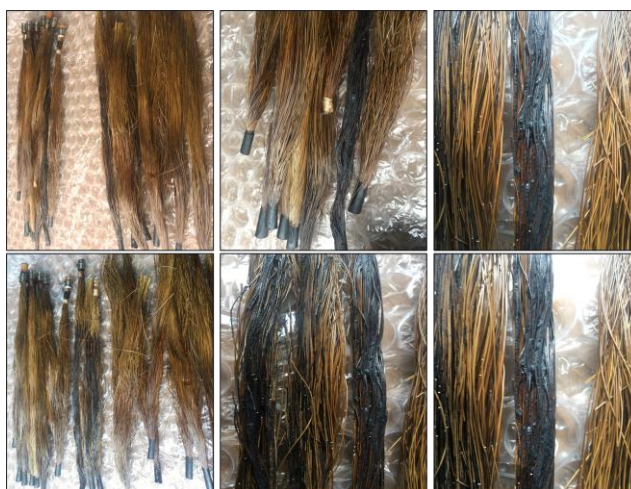
Figure 36. Fibers after being flooded with gasification water. Some fibers are completely coated with a black tar-like substance.
