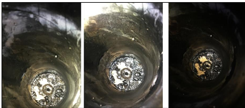
Figure 35. Pictures of the inside of module Old-1 after it was flooded with gasification water. There is a black solid material coating on the walls and at the bottom of the module vessel.
