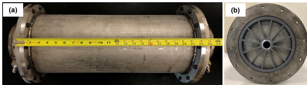
Figure 51. Photos of (a) \varnothing 8'' SW membrane module with membrane containing pEtC2 and (b) the end view of the element fitted in the module housing.
