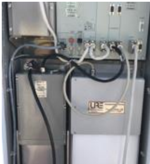
Ukraine Radiation Equipment (URE) installed in Aspect portal monitor
