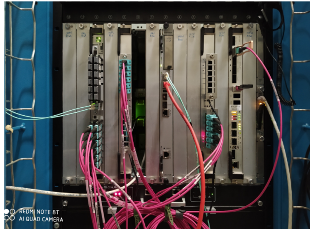
Figure-4: An ATCA shelf at the CERN TIF containing Apollo, Serenity, and DTH boards. Hahn’s team has established multi-gigabit communication between each of the boards in this crate.
