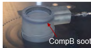
Sample loaded into base of Al shock tube, or into nozzle
