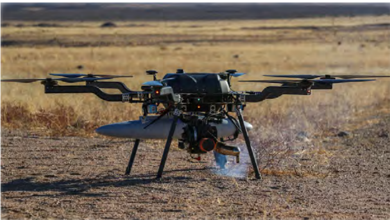
Payload will be flown by H6 drone to demonstrate multi-modal processing.
