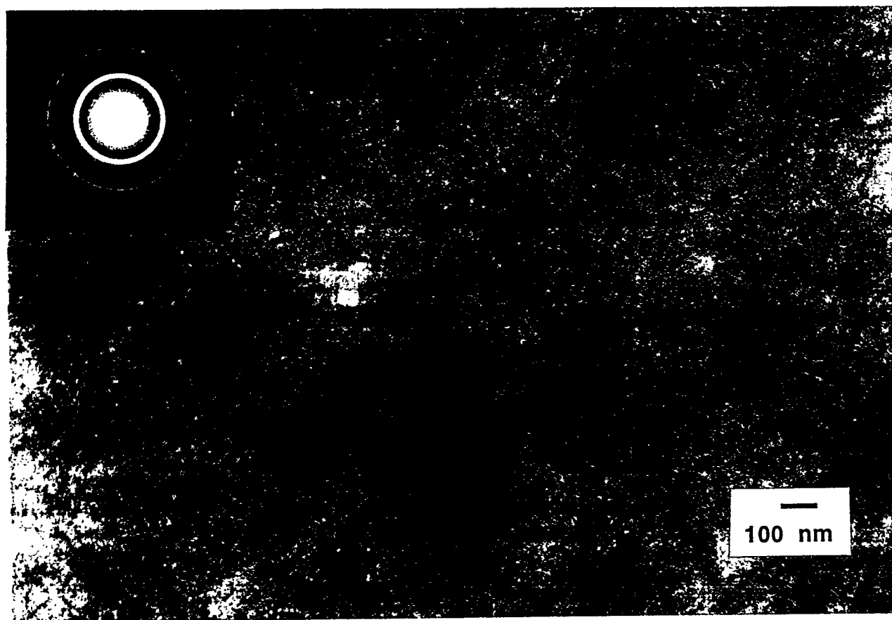
Fig. 2. Plan-view TEM image showing the microstructure and grain size distribution in diamond films grown from methane precursors in an argon plasma. The inset electron diffraction pattern indicates a random orientation distribution of the diamond grains.
