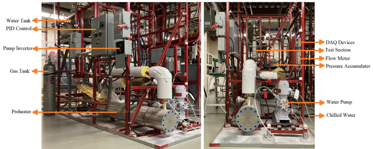
Fig. 1. Photos of the Flow Boiling Test Facility.
