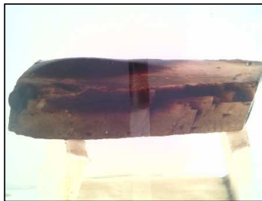
Figure 7. Oil-aged calcite plate in PW/16 after 24 hours. The plate was treated by 0.5 wt% Calimulse AOS solution for 7 days before aging in oil.
