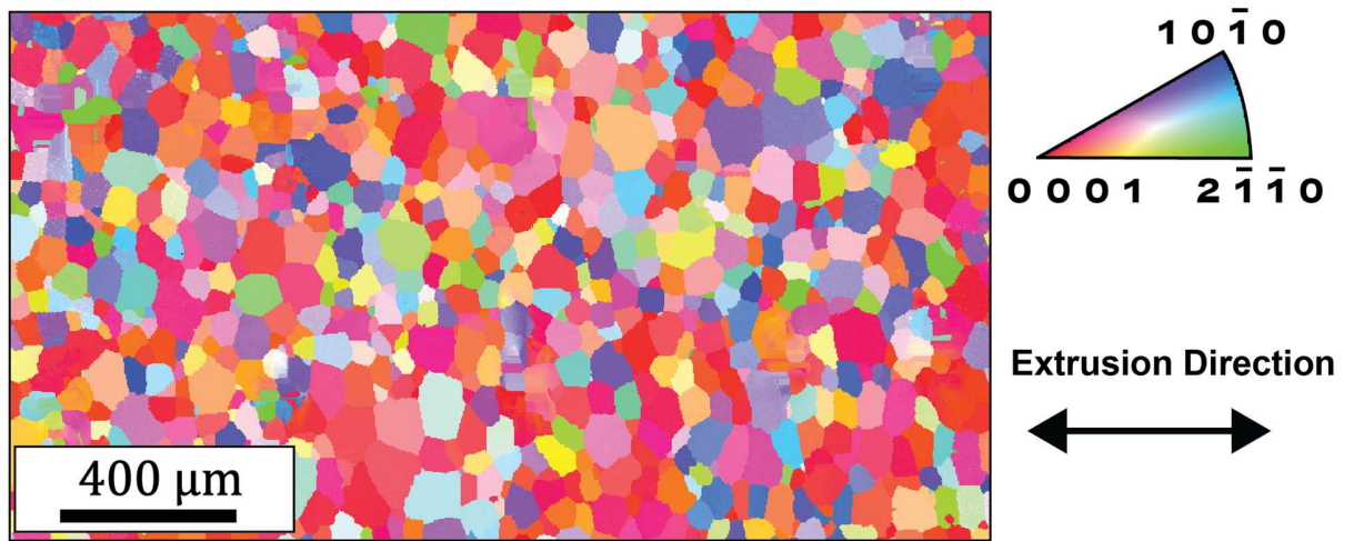
Figure 2: EBSD inverse pole figure map of extruded Mg-4Al (wt.%) with the average grain size of 55 μm.
