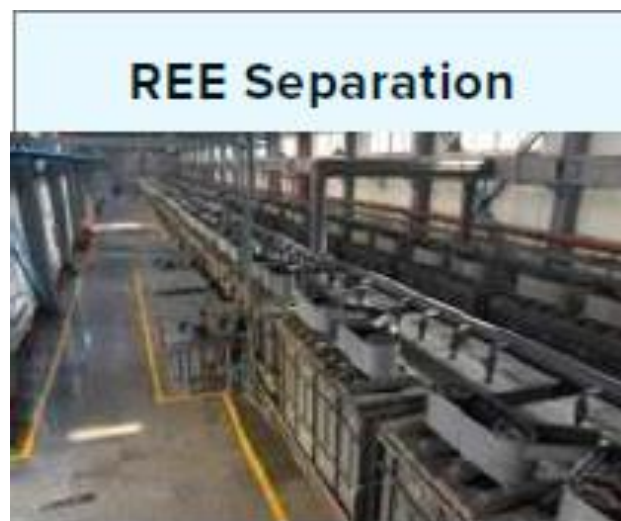
Figure 25. Neo Performance Materials Separation Facility Utilizing SX [25].
