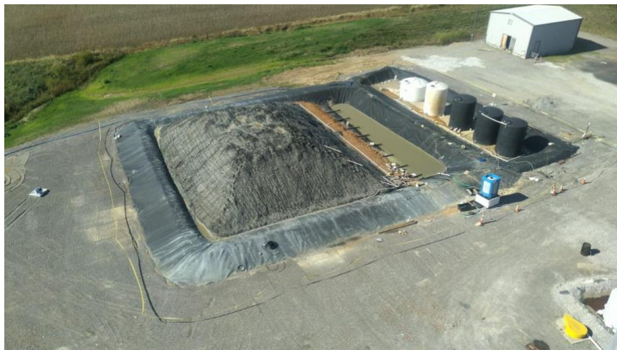
Figure 96. Test heap leach pad used to extract REEs from coal refuse.
