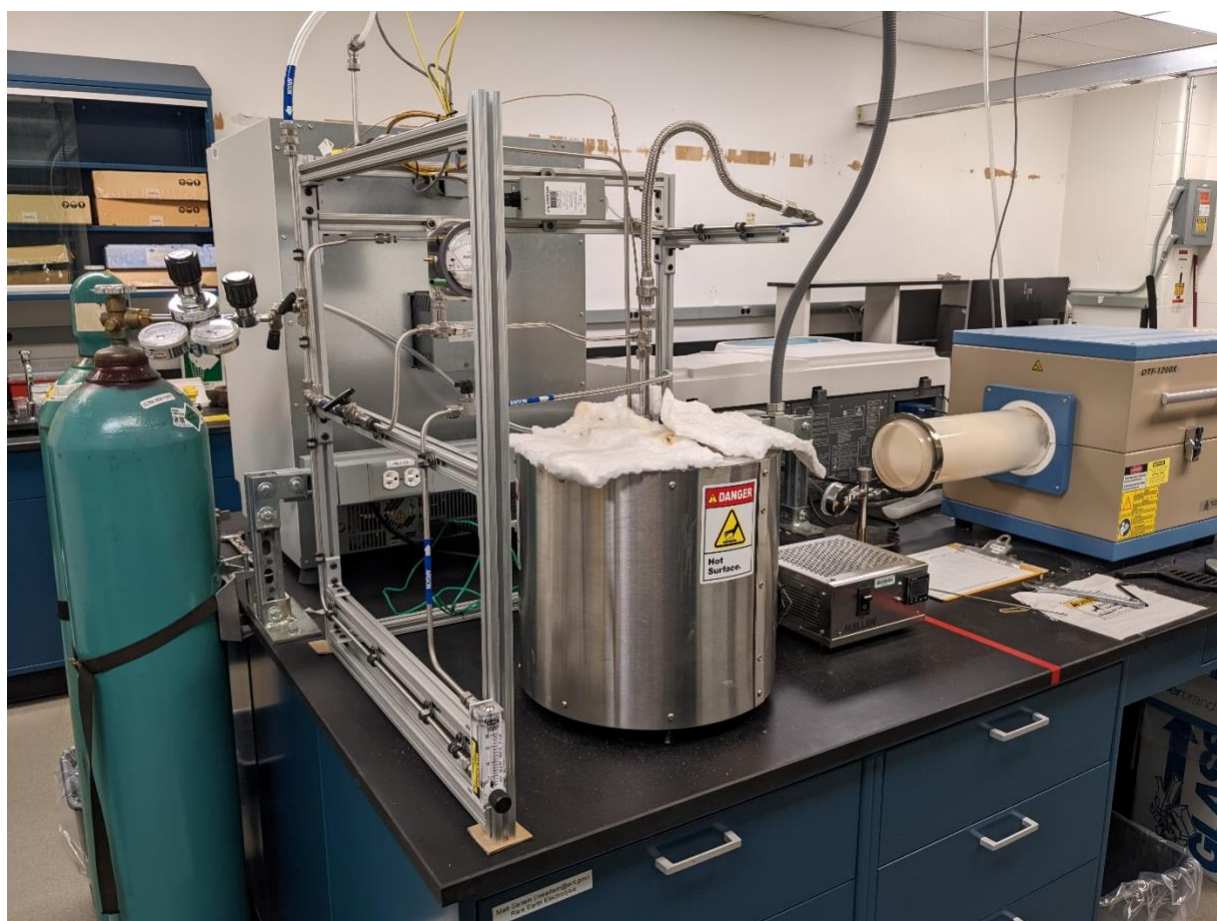
Figure 57. Lab scale molten salt EW cell used for testing.
