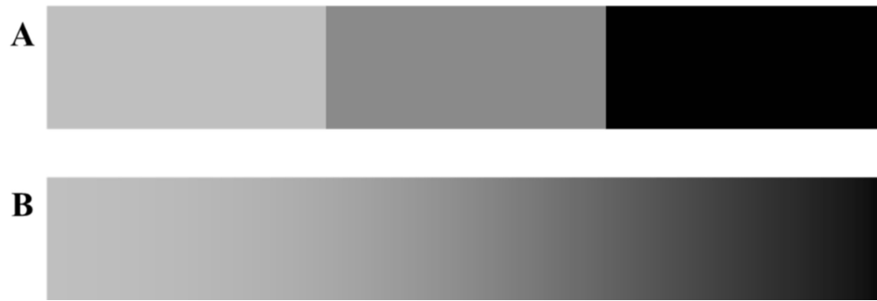
Figure 1. Graphical example of a stepwise FGM (A) compared to a continuous FGM (B).
