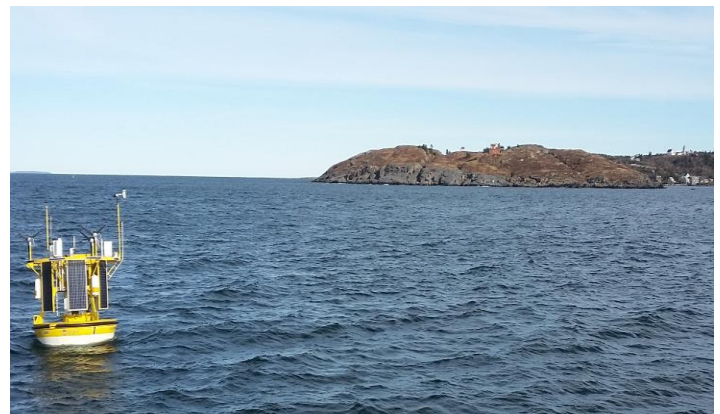
Figure 13 UMaine DeepCLiDAR buoy was deployed offshore Monhegan Island in December 2015 to collect hub-height wind speed. The buoy was validated by AWS True Power following the Carbon Trust Guidelines for Floating LiDARs It supplements 14 years of metocean data collected by an UMaine surface level buoy.
