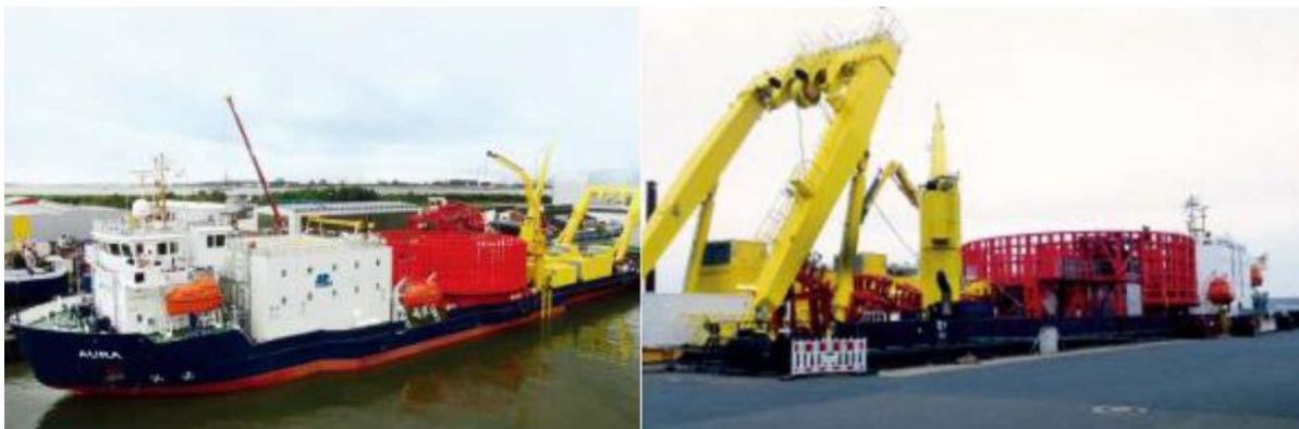
Figure 33 Cable laying vessel
