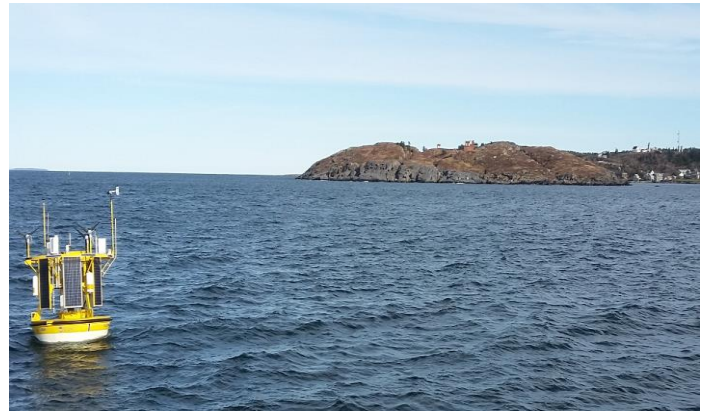
Figure 7 UMaine DeepCLiDAR buoy was deployed offshore Monhegan Island in December 2015 continues to collect hub-height wind speed. It supplements 14 years of metocean data collected by an UMaine surface level buoy.
