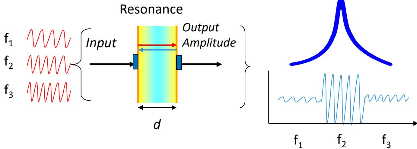
Resonance occurs when the **forward** sound wave and the **reflected** wave meet exactly in phase and **interfere**
