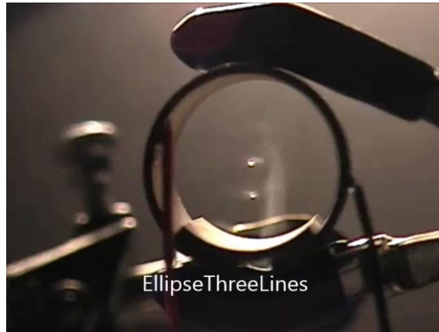
The video (real-time) shows the separation of mist from humidified air and concentrating the mist acoustically inside a hollow cylinder using sound. Once the mist is concentrated, it can be taken out of the system. Various types of implementation are possible and this is simply a proof-of-concept to show what is possible with sound.
