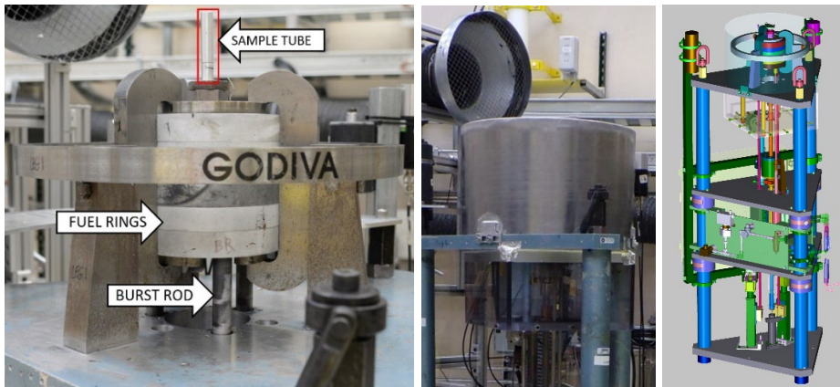
Fig. 1. (Left) Godiva IV with the ‘top hat’ removed and an aluminum sample tube inserted. (Middle) Godiva IV shown with the ‘top hat’ replaced. (Right) 3D CAD rendering of Godiva IV and associated mechanical drives and support structures.
