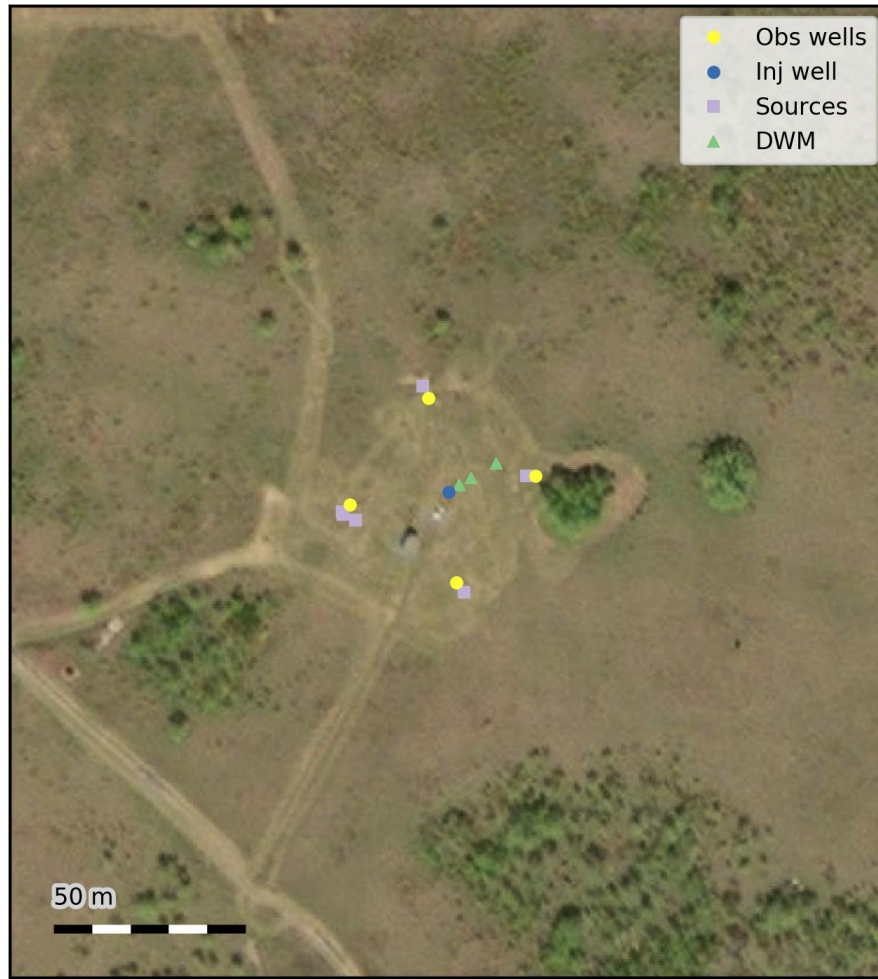
Figure A3-2: Injection and observations wells, along with AWD source locations, at the DFPS. Only DMWs 1-3 are shown (green triangles).
