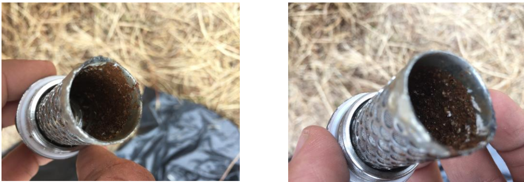
Figure 6-16: Two images of a strainer at different viewing angles, exposed at the end of all injection cycles. The orange/brown materials inside the strainer mesh are the solid debris separated from the injection water and accumulated behind the mesh in the strainer. The accumulation of this debris was confirmed during the experiments by a relatively large pressure drop through the injection manifold.
