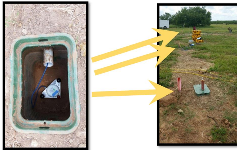
Figure A4-1: Tiltmeter vaults and tiltmeter installation. (left) The tiltmeter is the round can that is placed within the triangular plate. Leveling was performed by turning the black knobs at the corners of the plate. The blue data / power cable is threaded through the 2-inch PVC conduit to the remote Data-Acquisition-System electronics and power supply. (right) A closed tiltmeter vault in the foreground with a brick and a surveying target on top. Two additional vaults are in the background, and the data-acquisition-system electronics were located beside the stack of yellow shipping containers.
