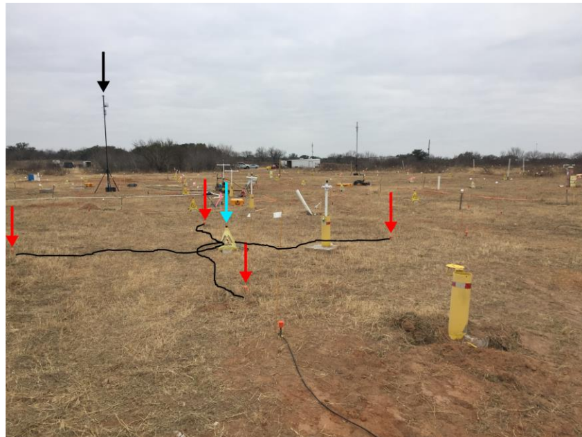
Figure 7-40: (a) Receiver deployment map. (b) An image of a set of four receiver rods, shown by four red arrows, and the associated wireless receiver, shown by a blue arrow, near DMW 4. The black lines show the wires that connected these receivers to the receiver rods. The wireless receiver communicated the data with the wireless tower, shown by the black arrow.
