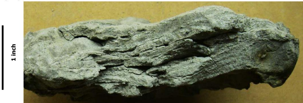
Figure A2-24: Photographs of muddy interdistributary-bay deposits in the DMW-1 core. (a) Mudstone with lenticular beds of siltstones and very fine-grained sandstone at 163.0-ft (49.7-m) depth. (b) Mud-dominated, planar-stratified section at 158.0-ft (48.2-m) depth. The corresponding core description is shown in Figure A2-6.
