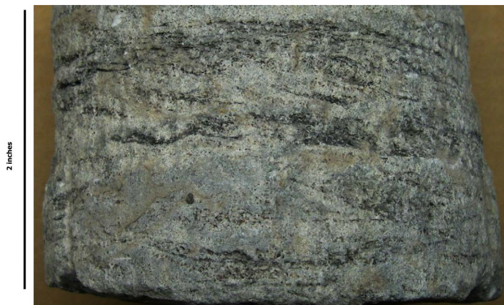
Figure A2-23: Photograph of ripple-stratified, fine-grained sandstone in crevasse-channel facies in the DMW-1 core at 187.0-ft (57.0-m) depth. The corresponding core description is shown in Figures A2-5 and A2-6.
