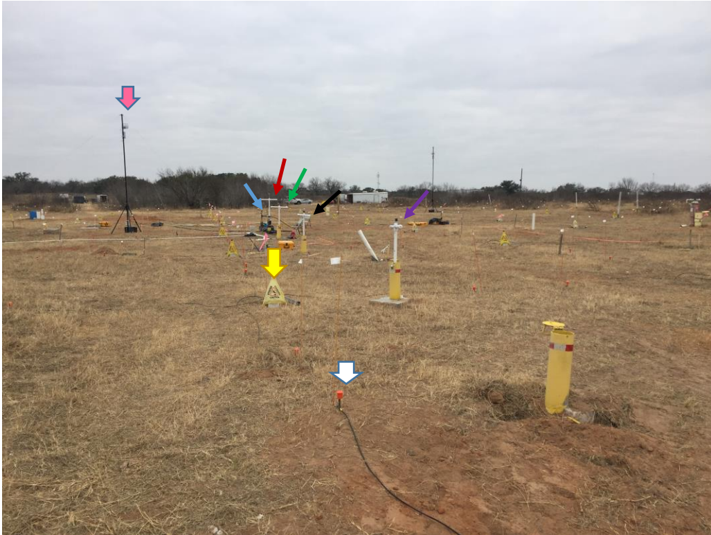
Figure 6-12: (upper) A panoramic view of the pump station; (lower) a close view of the survey area. (lower) Injection well and DMW 1 through 4 are pointed by blue, red, green, black, and purple arrow. 3-ft long receiver rods, shown for instance by the white arrow, were hammered to the ground for the CSEM survey and were wired to a receiver hub, shown by the yellow arrow, for data communication to the wireless antenna, shown by the pink arrow.
