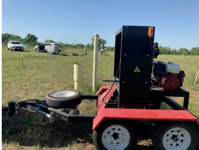
Figure A3-4: Accelerated Weight-Drop (AWD) source used at the DFPS.
