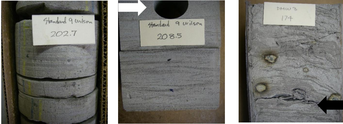
Figure 3-14: Representative cores from the DFPS Wilson-9 well (left two panels) and DMW 3 (right panel) are shown. Based on the predominance of cyclic mudstone beds and mud-draped ripples, we interpret this zone as tidal-flat facies. The two cores on the left had been used for prior geomechanical studies during the design phase of hydraulic fracturing at the DFPS with EAPs. Due to similarity between Wilson-9 well and DMW 3, the porosity/permeability and velocity data from Wilson-9 well were used for various modeling studies that were conducted as part of this project. White arrow in the center panel shows the location from which core plugs were extracted for geomechanical studies. The black arrow on the right panel indicates the position of the EAP containing fracture at ~ 175 ft. Core tags are 1 by 2 inches across.
