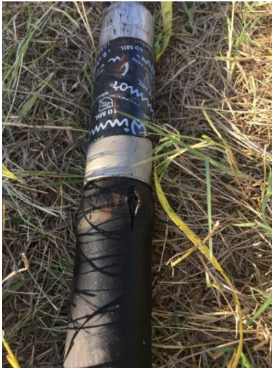
Figure 6-6: Puncture in the upper packer, which was encountered during the 9/22 injection. This was remedied by the placement of a bridge plug in the injection well below the perforation zone on 9/23.
