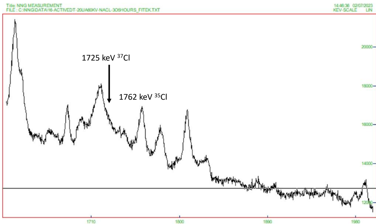
Fig. 9: Un-background subtracted gamma-ray spectrum from DT (14 MeV) neutrons on NaCl sample showing the background in the region of the ^{35}\text{Cl} and ^{37}\text{Cl} peaks.
