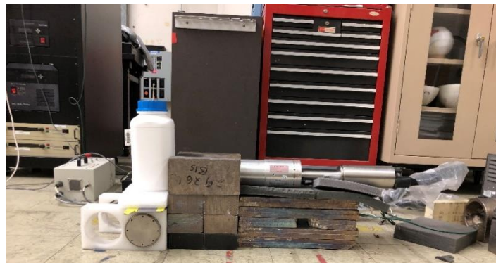
Fig. 5: The experimental setup consists of (from left bottom to right top) borated polyethylene, a neutron source, a sample separator and the KCl sample, bismuth bricks, a collection of foam to prop the HPGe detector up, and finally the HPGe detector. The HPGe detector was about 10 cm from the edge of the samples.
