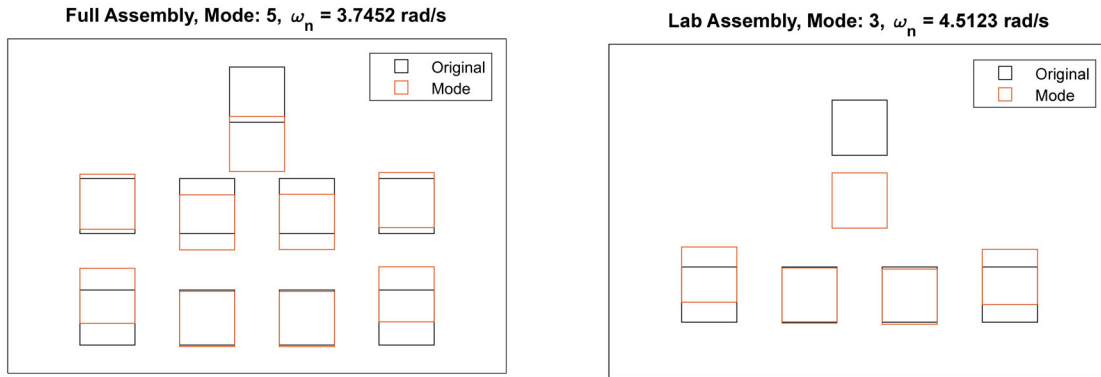
Figure 7: Mode Shapes of the (a) S+TS+V system and (b) S+TS system
