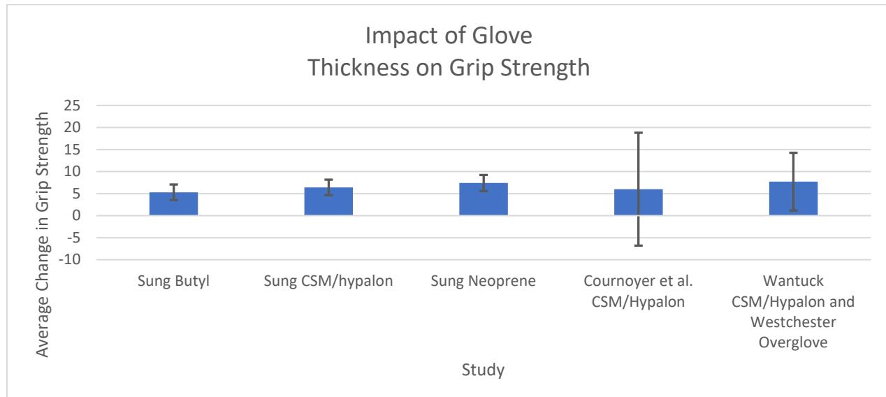
*Note.* The average change in grip strength force for each study element (each using varied glove thicknesses). The error bars shown represent the standard error associated with the study.
