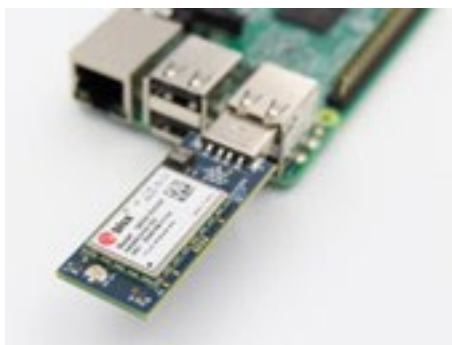
Figure 23: Hologram Nova cellular modem plugged into a Raspberry Pi.
