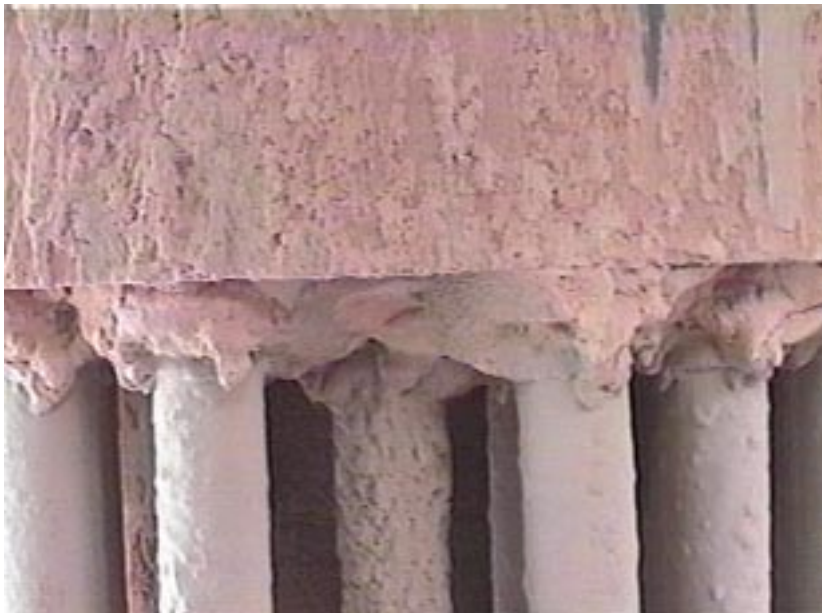
Figure 4. This photograph shows the typical ash deposits formed around the mounting locations on the top filter plenum (May 18, 1998).
