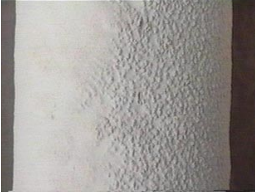
Figure 3. Typical smooth filter cakes observed on the bottom filter plenum on May 18, 1998.
